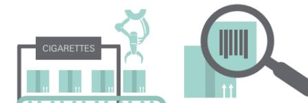
Serialization and aggregation of products throughout the manufacturing process using Codentify, to embed unique information
